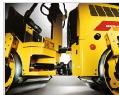
Maintenance-free articulated joint and steering cylinder.
